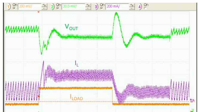
Figure 21. Load Transient 150mA to 400mA, V_{IN}=3.6V , t_{RISE}=t_{FALL}=100ns , 5µs/div.
