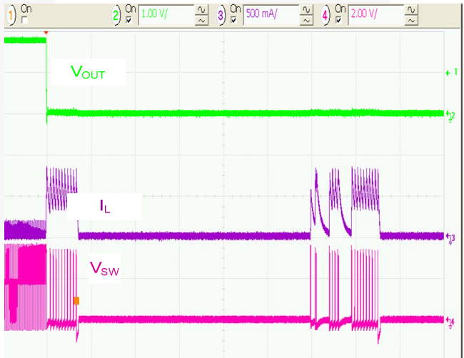
Figure 16. Metallic Short Applied at V_{OUT} , 50μs/div.
