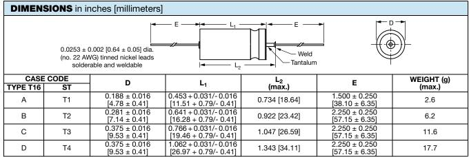
For insulated parts, add 0.015" [0.38 mm] to the diameter. The insulation shall lap over the ends of the capacitor body.
