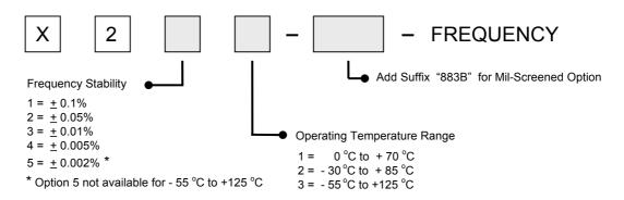
EXAMPLE: X243 - 883B - 4.000 MHz = 14 Pin Package with "X" Pinout, CMOS,  $\pm$  0.005% over -55 °C to +125 °C, Mil-Screened, and 20.000 MHz
