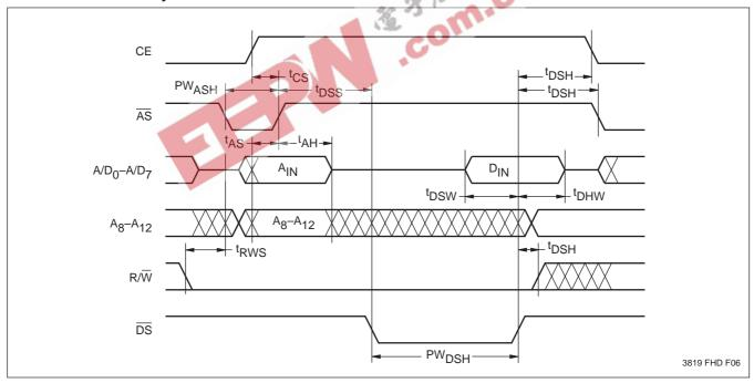
Note: (4) t<sub>WC</sub> is the minimum cycle time to be allowed from the system perspective unless polling techniques are used. It is the maximum time the device requires to automatically complete the internal write operation.
