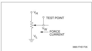
**Notes:** (1) Absolute Linearity is utilized to determine actual wiper voltage versus expected voltage =  $(V_{W(n)}(actual) - V_{W(n)}(expected)) = \pm 1$  MI Maximum.
