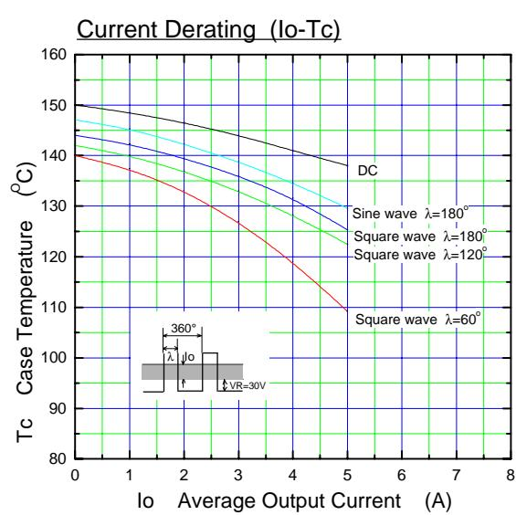
$\lambda$ :Conduction angle of forward current for each rectifier element
