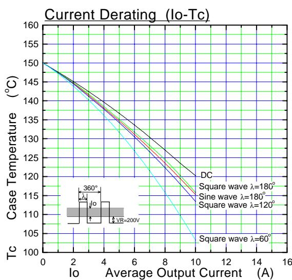
$\lambda$ : Conduction angle of forward current for each rectifier element
