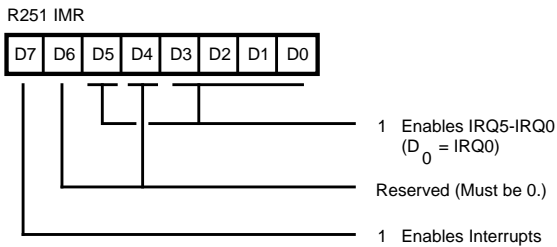
Figure 33. Interrupt Mask Register (FB H : Read/Write)
