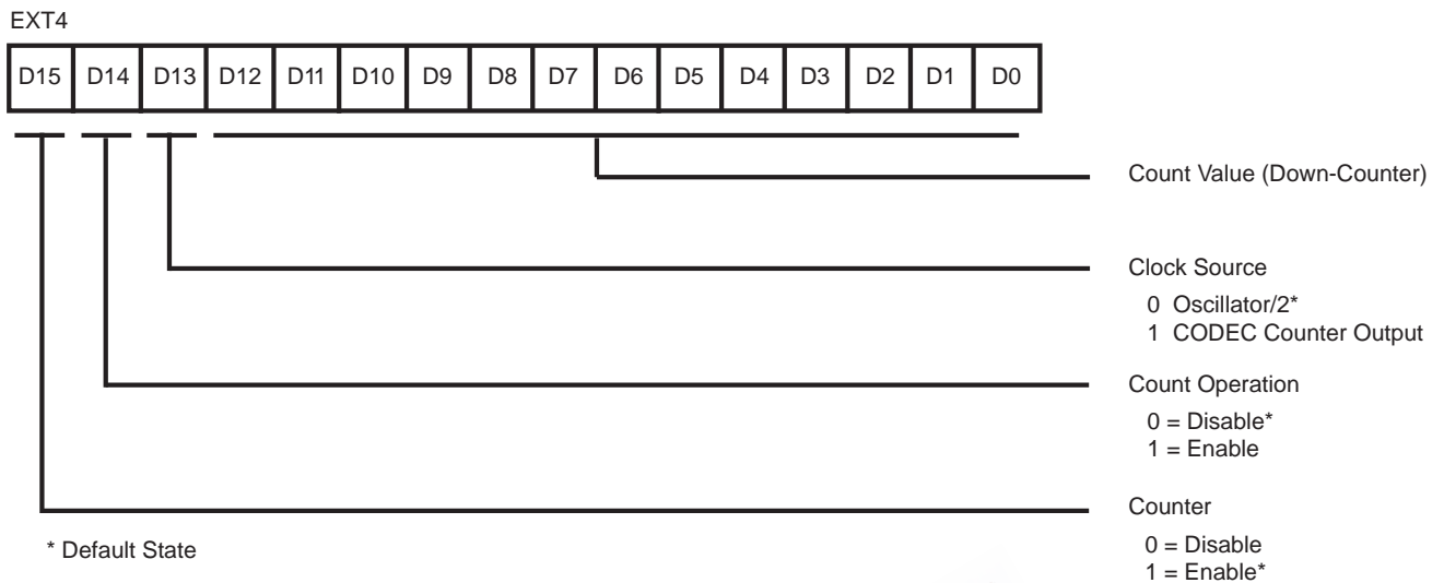
Figure 33. CODEC Timer Register
