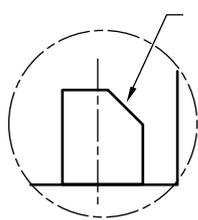
DETAIL A PIN 1 LEAD SCALE 50:1
