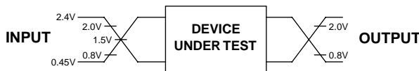
During AC testing, inputs are driven at 0.4V and 2.4V levels. Unless otherwise specified, switching times are measured from the 1.5V level of DCLK to the 0.8V or 2.0V levels at the input/output.
